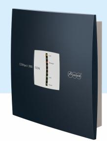
Compact ICT system with up to 4 external lines (via ISDN), up to 8 subscribers (ISDN, IP, analogue) and ability to expand by one ISDN port or 2 analogue subscriber ports
