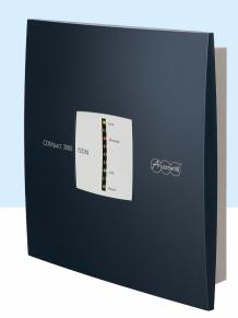
Compact ICT system with up to 4 external lines (via ISDN), up to 8 subscribers (ISDN, IP, analogue) and ability to expand by one ISDN port or 2 analogue subscriber ports
