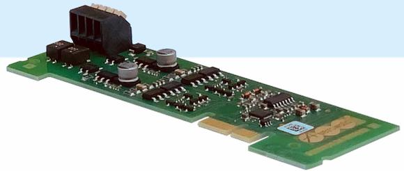
Expansion for COMpact 3000 with two internal analogue ports for analogue terminals
